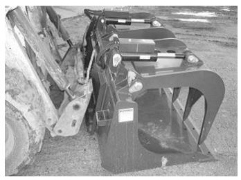
3. Drive the loader to the rear of the attachment. Put the loader quick attach coupler into the attachment mounting bracket.
