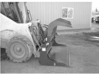
3. Activate the loader's auxiliary hydraulics to open and close the grapple in order to pick up and move debris/objects.
