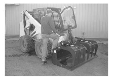
1. Use the step, safety treads, and grab handles to get on and off the loader and attachment.
